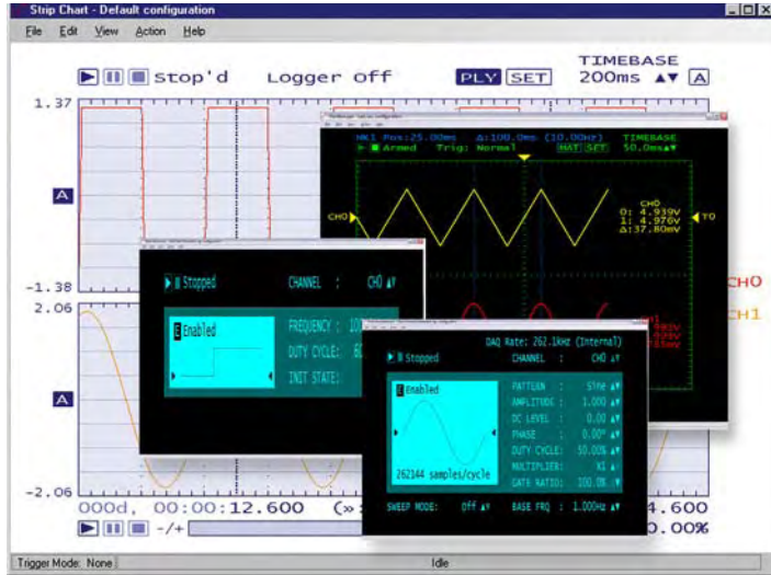
TracerDAQ provides four virtual instrument applications used to graphically display and store input data.
