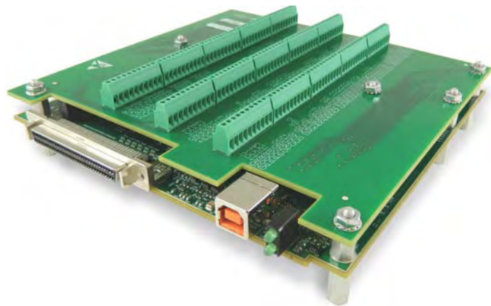
USB-2637 connected to TB-103 screw-terminal board.
