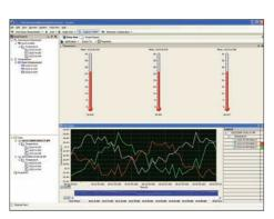
Encore can display channel data in several ways including meters, gauges, tanks and graphs
