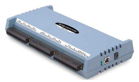
The USB-2416 Series offers high-resolution voltage or thermocouple measurements along with digital I/O. Analog output functionality is available with the USB-2416-4AO.
