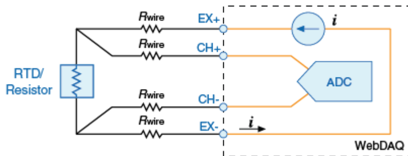
Figure 9. 4-wire resistance and RTD circuitry
