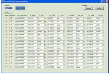
HART Device Simulator (called HDS) is the HART device simulation software developed by ICP DAS. It can be used to simulate multi HART slave devices simultaneously to exchange data with HART master device by using ICP DAS HART converter (like: <u>I-7567</u> / <u>I-7570</u> / <u>I-7547</u>) connected to any COM port (USB / 232 / 485 / Ethernet). By this way, users can develop or verify the HART master program without any HART slave device.
