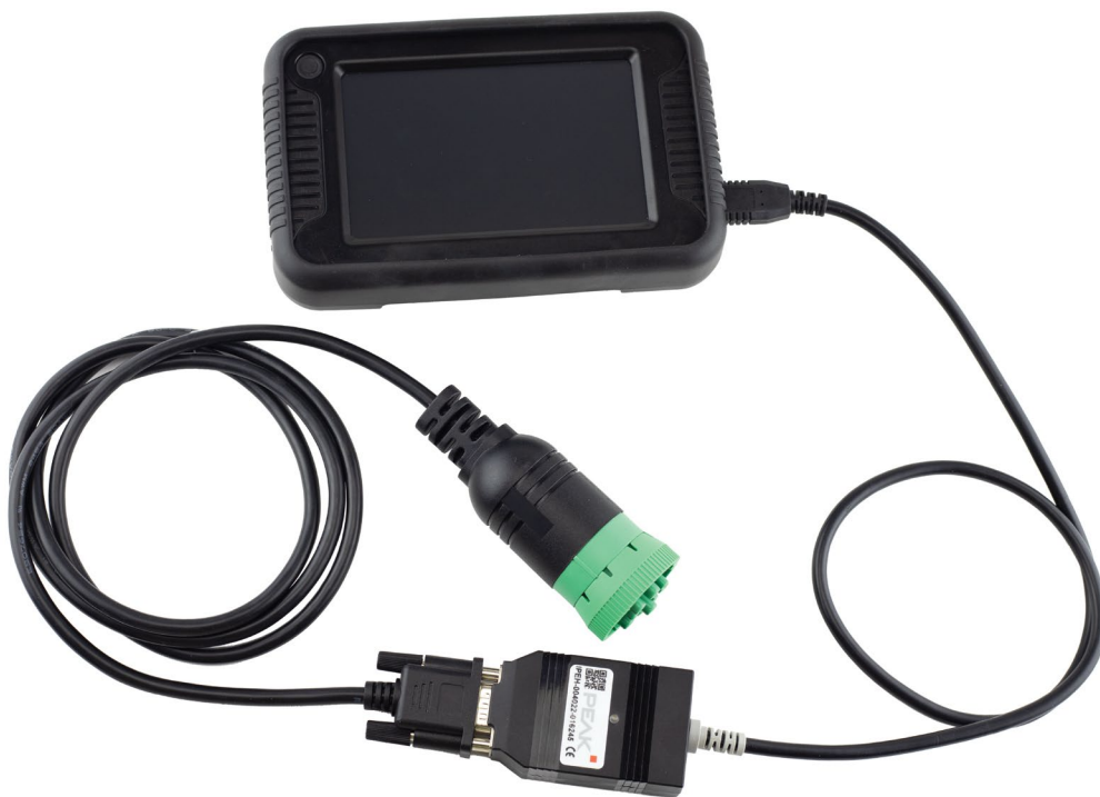
CAN Connections are made by connecting CAN converter to USB port. Diagnostic cable is then plugged into the 9-pin DIN connector and plugged into the vehicle.
