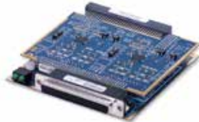
DNF-series FLATRACKS use DNF-series boards such as this DNF-1553-553.
