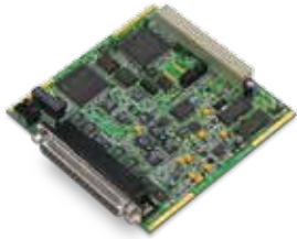
DNA-series boards such as this DNA-AI-207 are used with Cube, DNA-series and UEINet chassis.
