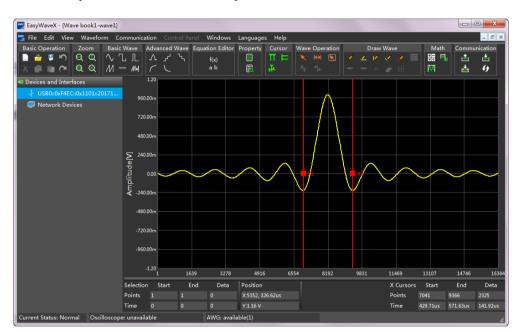
EasyWaveX is an arbitrary waveform software platform that supports waveform creation and editing. It features manual drawing, as-well-as line, equation, and coordinate editing modes. It is also a convenient way for users to edit their own arbitrary waveforms.
