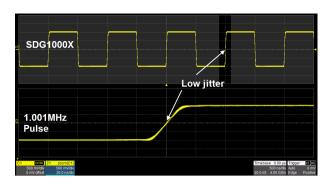
When a Pulse waveform is generated by a common DDS generator, there will be a one-clock-jitter if the sampling rate is not an integer-related multiple of the output frequency. SDG1000X EasyPulse technology successfully overcomes this weakness in DDS designs and helps to produce low jitter Pulse waveforms.
