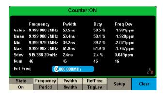
High precision Frequency Counter with an input frequency range of  $0.1~\text{Hz}{\sim}200~\text{MHz}.$
