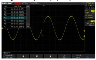
Playback history waveform to observe unusual events and locate the source quickly through the cursor or measurements, located on the keyboard Panel, this function is easily enabled. Segmented memory collection will store the waveform into multiple (up to 80,000) memory segments, each segment will store a triggered waveform and dead time information
