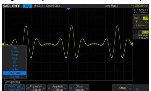
The SDS1000X+ has a built-in 25 MHz function / arbitrary waveform generator (standard), including 10 built-in waveforms plus 4 ARBs. The arbitrary waveforms can be accessed and edited by the EasyWave PC software
