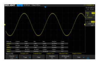
Parametric statistical functions to display any parameters of the five measurements: current, average, minimum value, maximum value, and the standard deviation. The measurement count is also displayed. The maximum number of parameters that can be measured and simultaneously analyzed statistically is five. Supports Gating measurements, Math measurement, History measurement, Ref measurement.
