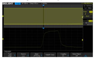
Using hardware-based Zoom technologies and record length of up to 14 Mpts, users are able to use a higher sampling rate to capture more of the signal, and then quickly zoom in to focus on the area of interest
