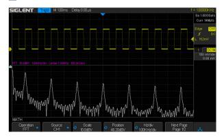
In addition to the traditional (+, -, X, /) operation, SDS1000X/ SDS1000X+ oscilloscopes supports FFT, integration, differentiation, and square root operations.
