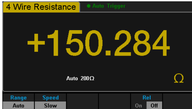
Diagram 2- 15 4-Wire Resistance Measurement Interface
