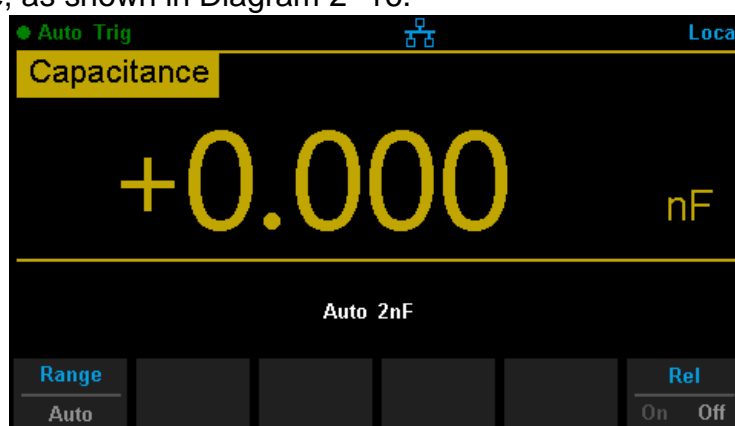
Diagram 2- 17 Capacitance Measurement Interface
