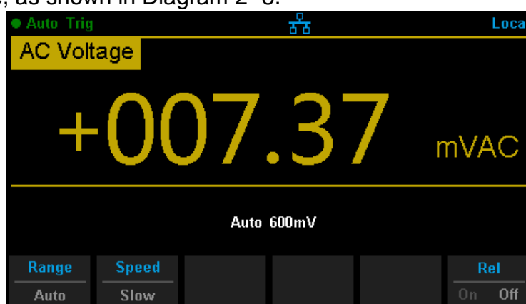
Diagram 2- 8 AC Voltage Measurement Interface
