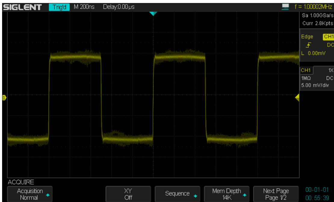
Figure 17 With Random Noise, Normal Mode
