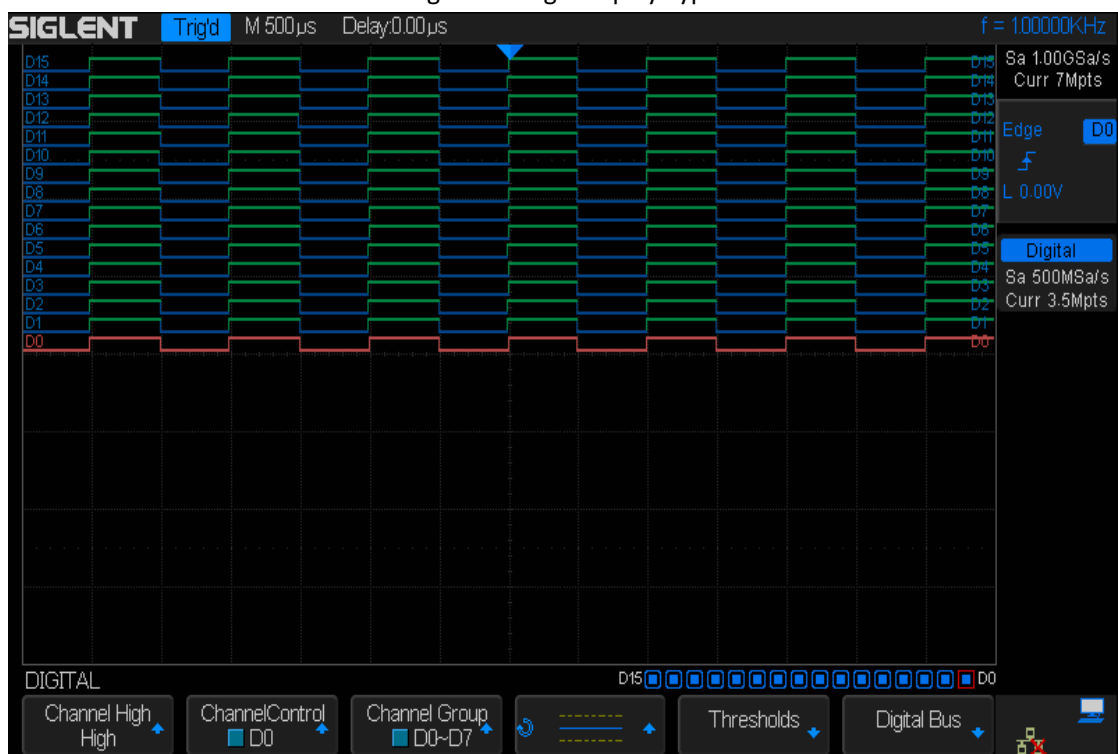
Figure 40 High Display Type
