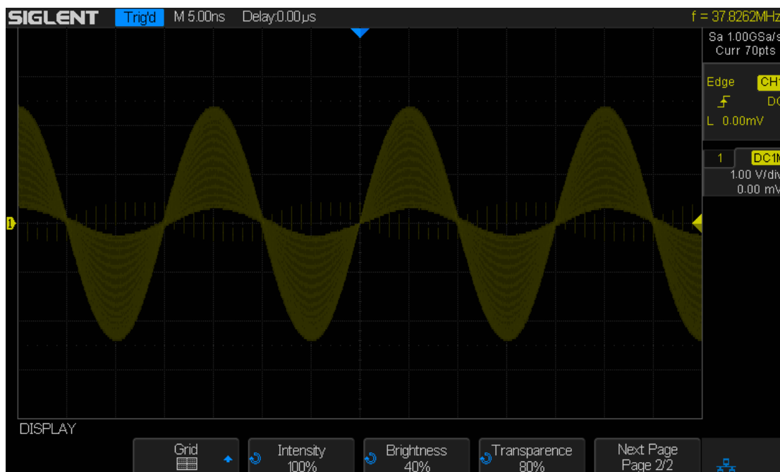
Figure 62 Intensity Set to 100%
