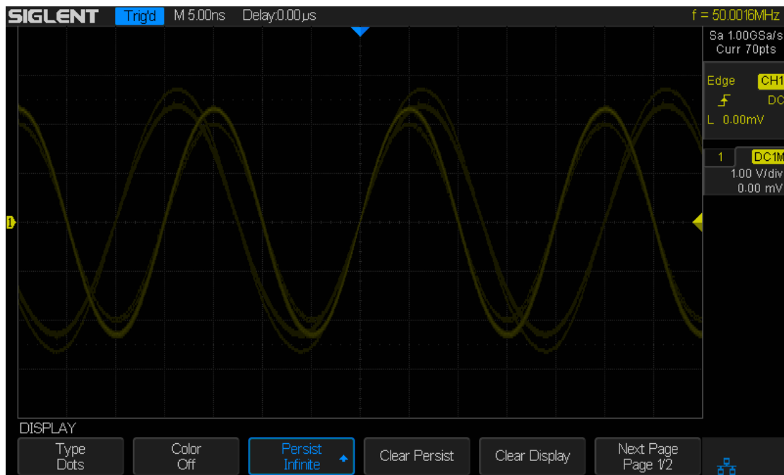
Figure 61 Persist Set to Infinite
