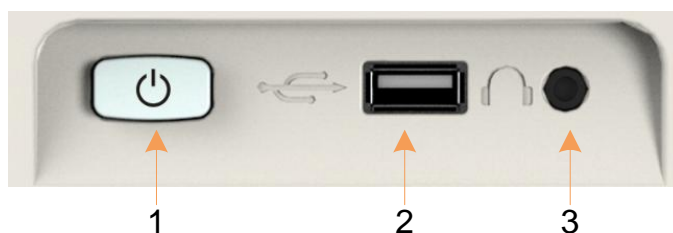
Figure 1-9 Front Panel Connectors (1)
