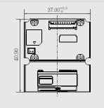
53.00mm W x 40.90mm D x 15.20 mm H (Wide board with three mounting areas and connected by molex cable. The engine is mounted on the board.) 37.00 mm W x 40.90 mm D x 15.20 mm H (Wide board with one mounting area and connected by molex cable. The engine is mounted on the board.)
