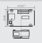
37.00 mm W  $\times$  23.40 mm D  $\times$  12.00 mm H (Narrow board with one mounting area and connected by molex cable. The engine is separated.)
