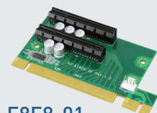
RC-E8E8-01 Riser Card with 2x PCIe8 Slots Interface: 1x PCIe16 + 1x PCIe1 Expansion: 2x PCIe8 Dimension: 111.3 x 60.5 mm
