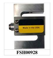
**Model:** LSB350, 3000 lb, Tension & Compression Load Cell, Standard, Material - 17-4 PH S.S., 1/2-20-Thread, 28 Awg 6 Conductor Shielded Retractile PVC Cable, 10 ft Long
