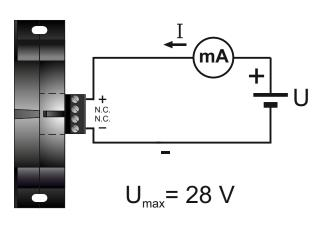
A maximum voltage supply of 28 V can be connected directly to the loop 4 – 20 mA of the T201DC100.
