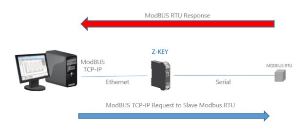
The Master (client) Modbus TCP-IP request a modbus register by ethernet, then the Z-KEY convert the request to the serial Modbus RTU slave, the Modbus RTU response is also retranslated in Modbus TCP to the Master.
