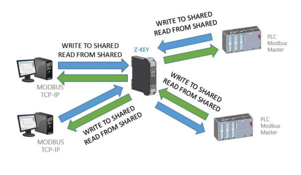
The Z-KEY shared memory can be freely read and written from Ethernet or/and from the serial ports. The Shared memory registers must be defined before with the setup TAG section.
