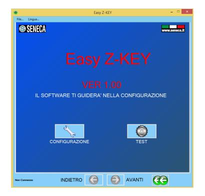
Connect Z-KEY to a PC with a standard micro USB cable, power up the Z-KEY and Click on "TEST" to obtain the actual IP address:
