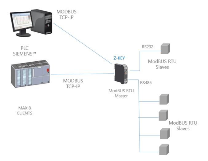
Also a remote communication through internet with multiple clients is possible, with the gateway configuration the tags are visible through the internal webserver:
