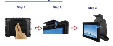
1.Slide the latch to open the hook
