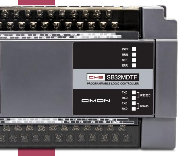
CIMON's CM3 Micro-S brick PLCs are tailored for compact, standalone machine control and remote automation tasks, offering versatile communication and I/O functionalities. They can accommodate up to 36 I/O points and have built-in features, including Ethernet connectivity, high-speed counting (HSC), pulse-train output (PTO) motion control, proportional-integral-derivative (PID), and analog I/O support.
