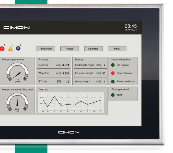
CIMON's Xpanel human-machine interfaces (HMI) facilitate interaction between humans and machines. They undergo rigorous testing for high levels of shock, vibration, and temperature resilience. These devices operate efficiently in industrial environments and are packaged with many communication interfaces.
