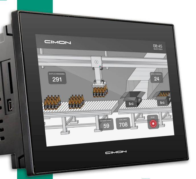
CIMON's Xpanel human-machine interface (HMI) facilitates interaction between humans and machines. They undergo rigorous testing for high levels of shock, vibration, and temperature resilience. These devices operate efficiently in industrial environments and are packaged with many communication interfaces.
