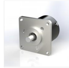
MB-FL6 Flange adapter, 2.5" square with 1.25" male pilot
