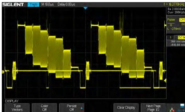
256-level intensity grading display on waveform.
