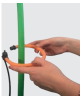
First generation Rogowski sensor, output 100 mV/kA, 50-60 Hz, Ø 115 mm
