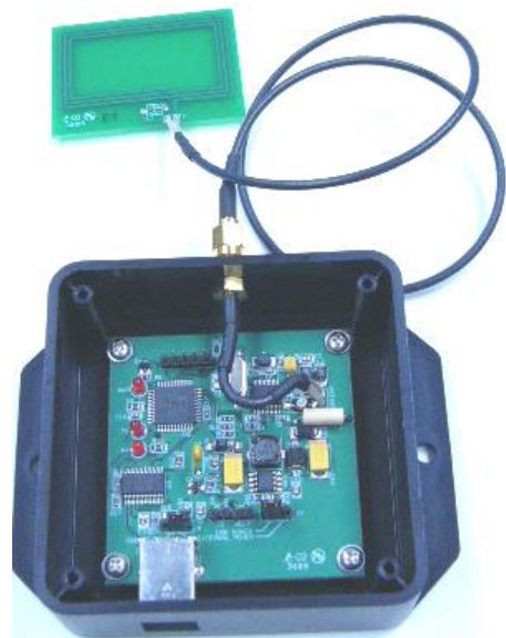
Reader with external Antenna
